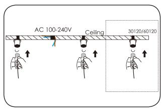
**6** Screw the suspension cable to the ceiling fixing.
