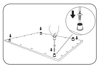
3 Screw the suspension panel fixing to the LED Panel.
