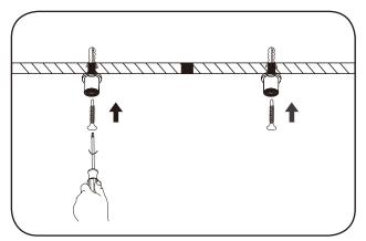
1 Insert the wall plugs into the ceiling and secure the suspension surface fixing to the ceiling.
