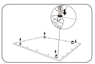
4 Screw the suspension cable to the LED Panel.
