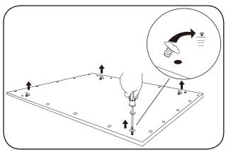
2 Unscrew the highlighted screws from the four corners of the Panel.
